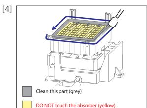
Use the cleaning stick to clean around the rubber part of the capping unit to remove the ink deposits and dust.
