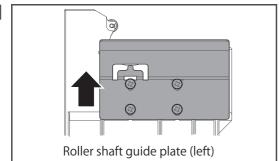
Do the same for the left media holder to slide up the roller shaft guide plate as far as it will go and tighten the screws.
