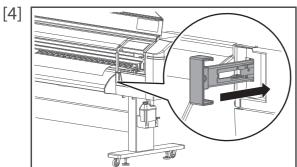
(To cancel the individual pressure rollers) Push the media feed lever back to the original position to lock the pressure rollers.
