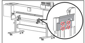
(When looking from the rear side of the printer) Use the screwdriver to loosen four screws securing the roller shaft guide plate to the right media holder.
