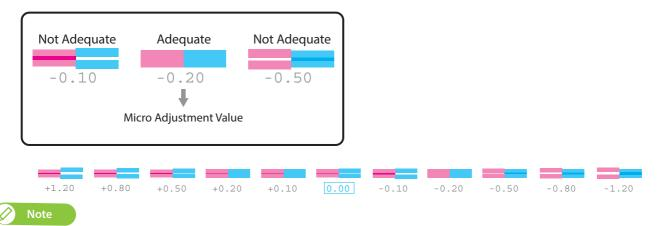
Once an appropriate micro adjustment value has been saved, the value will be the baseline value from the next time to be printed in the center of the pattern.
