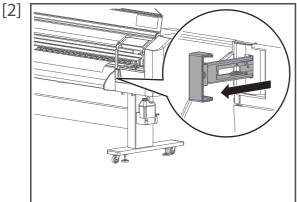
(To cancel the individual pressure rollers) From the front side of the printer, pull the media feed lever towards you as much as possible to release the pressure rollers.
