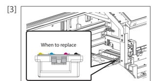
Check the absorption material for the flushing box.
