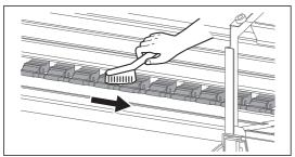
Brush off dusts on the pressure rollers with a soft brush.
