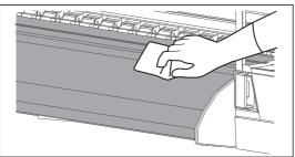
Use a soft cloth or paper towel slightly dampened with ethanol to clean off the ink on the platen, media guide and edge holders.
