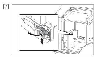
Press the cutter cap lightly, return Cutter holder to its initial position.
