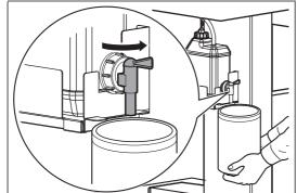
Open the waste ink valve and drain waste ink into the container.
