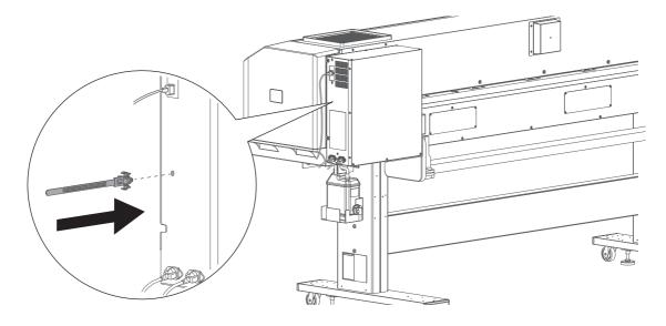
$[3] \qquad \text{Use the cable tie to secure the Ethernet cable to the printer.}$
