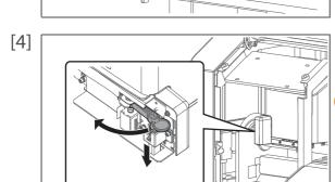
Press the cutter cap lightly, turn Cutter holder in the direction as illustrated below.
