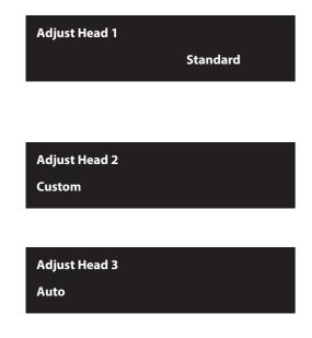
The Standard option performs the head alignment for the print mode saved in the currently selected user type.
