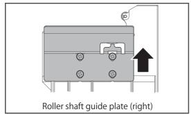
Slide up the roller shaft guide plate as far as it will go and tighten the screws.
