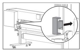
You can access to the media feed lever from the rear side of the printer.
