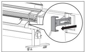
From the front side of the printer, pull the media feed lever towards you to release the pressure rollers.
